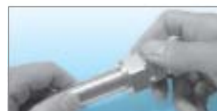
5. Insert the tubing into the Hy-Lok two ferrule tube fittings and confirm that the line made by the tube marker is not visible. The tube is now properly inserted and the fitting can be tightened.
