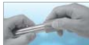
2. After inserting the tubing, press the marker lever and rotate the tube marker.
